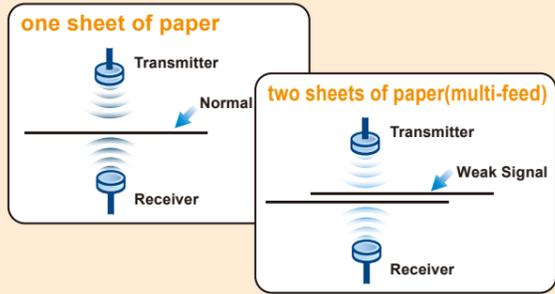
The PS3140U scanner prevents multi-feeds by checking the thickness of documents and detecting overlapping pages with the built-in ultrasonic multi-feeds detection capability. Users will be warned when a multi-feed is detected.
